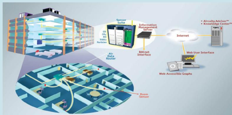
The air samples are transported to the central set of sensors for the analysis through a common air and data bus, which is manufactured with nanotechnological materials that provide inert properties which minimize the chemical absorption and maximize the transport of particles.
